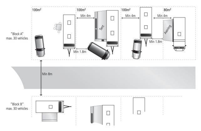
The figure shows the recommended distances between the blocks of a camping site and the recommended minimum distances between the different camping vehicles/units (from Ref.1).
